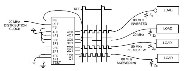
Figure 9. Board-to-Board Clock Distribution
