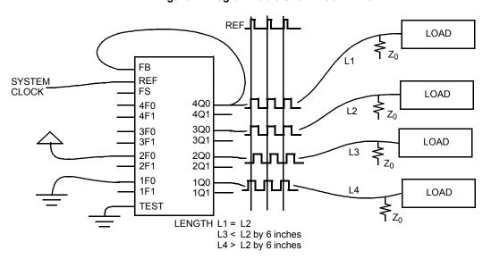
Figure 4. Programmable Skew Clock Driver
