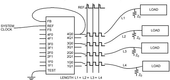
Figure 3. Zero Skew and Zero Delay Clock Driver
